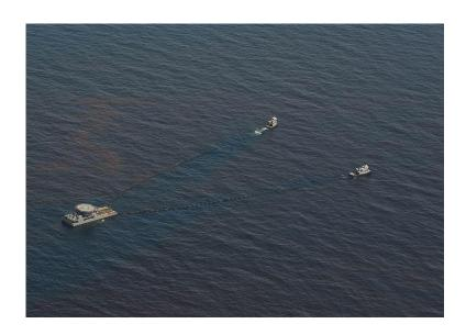
Special boats known as skimming boats also began working to clean up the spill. These boats use brushes, belts, and machines to separate oil from the water. They skim the oil off the water's surface and collect it.
